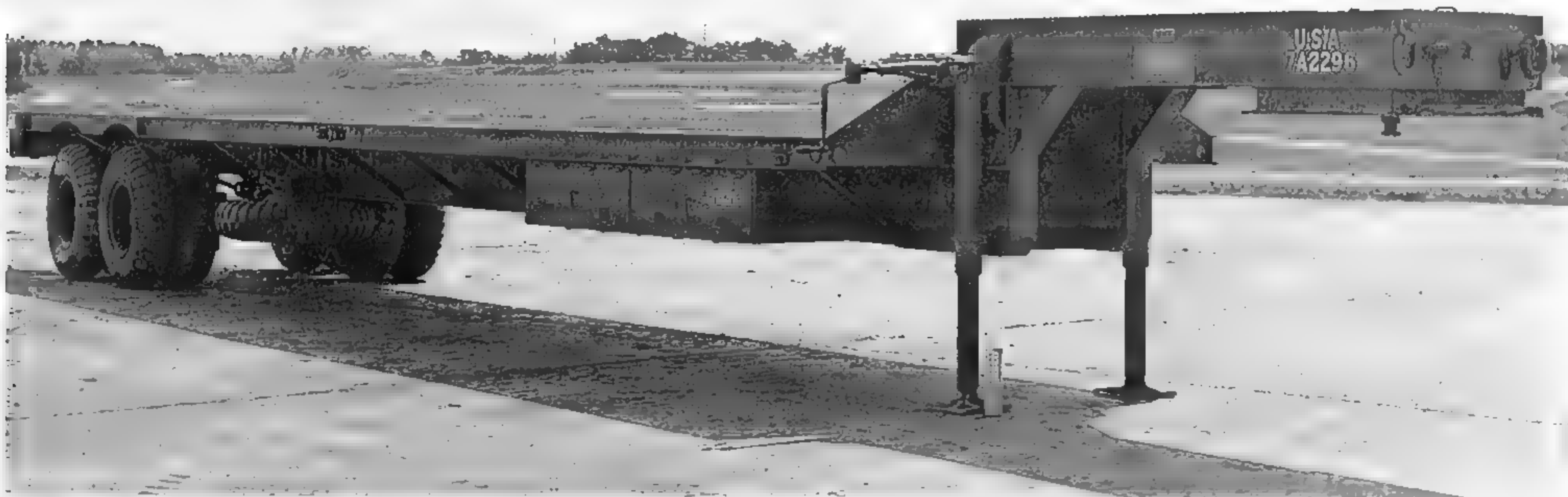
This factory-new M270A1 was photographed while being tested by the Armor and Engineer Board. The M269 series trailers were identical, but shorter. (Photo courtesy of the Patton Museum)
